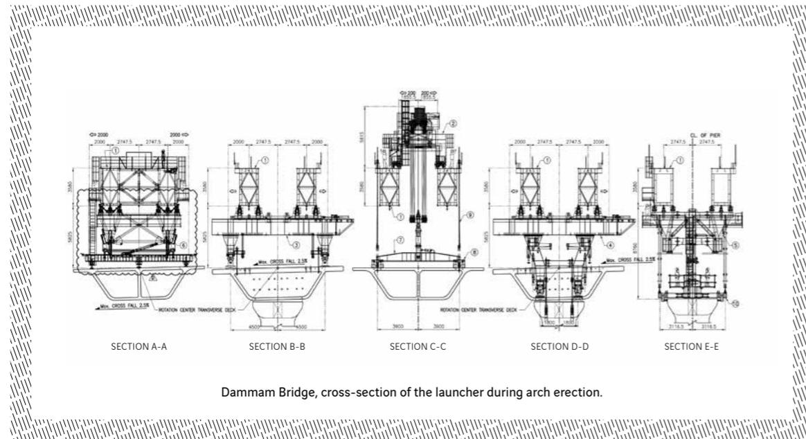
Dammam Bridge, cross-section of the launcher during arch erection.
